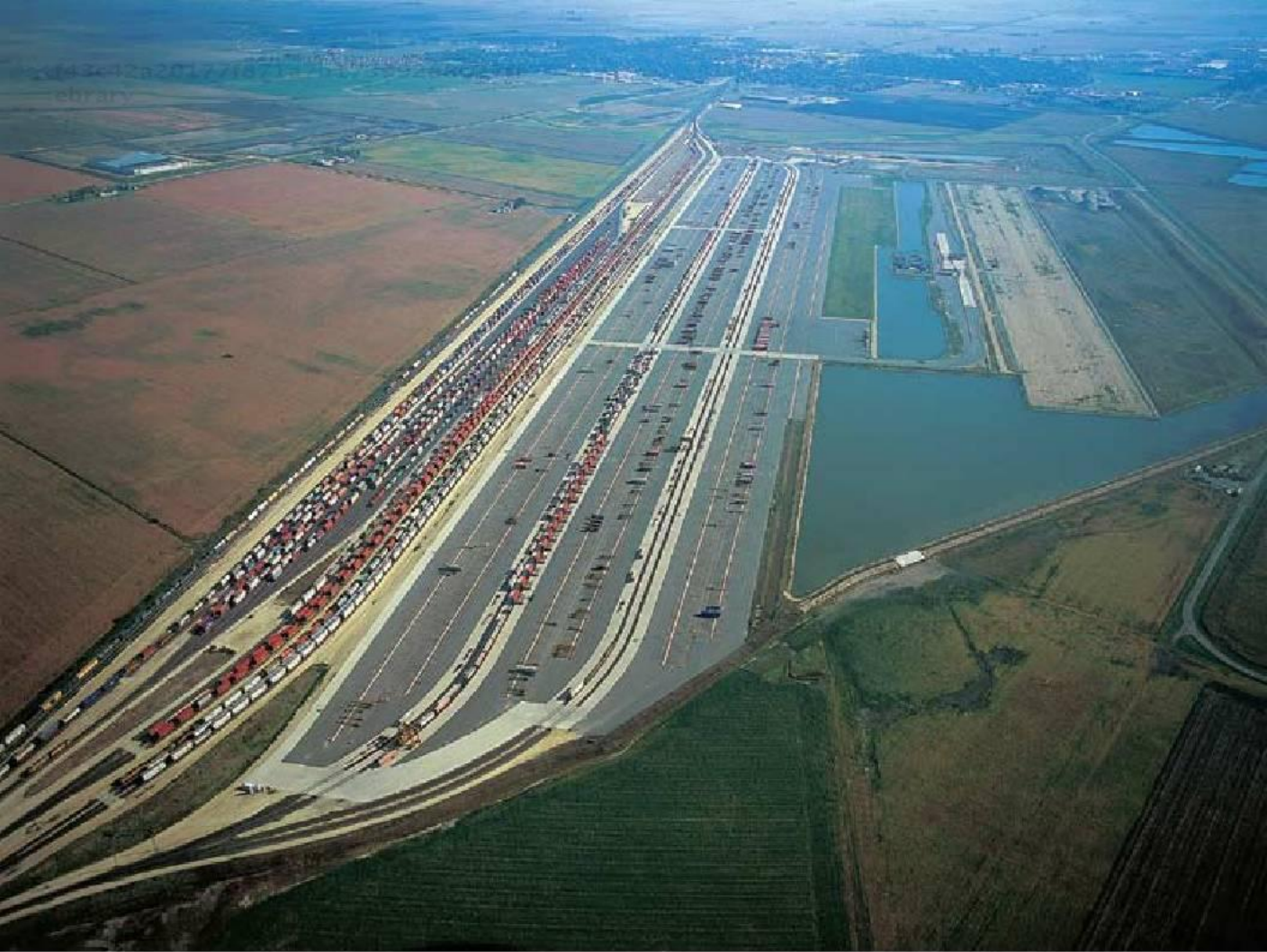
20—Global III Intermodal Terminal, Rochelle, Illinois, about eighty miles west of Chicago Union Pacific Railroad's facility was completed in 2003. It features a ten-lane automated gate system and processes over 7,200 containers daily.
